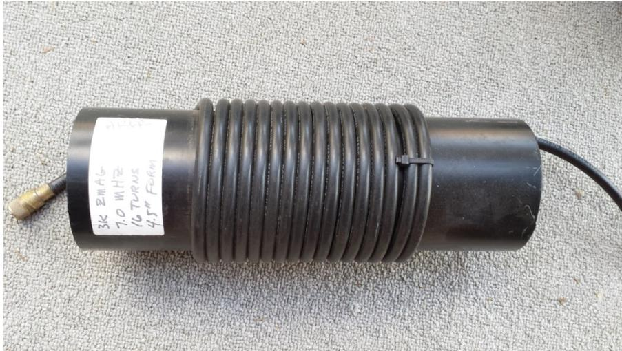
This higher power BALUN or UNUN utilizes mil-spec coax cable for the windings. Available wired as a BALUN (Palomar # TCC-40B) with +/- output terminals or as a UNUN (Palomar # TCC-40U) with PL-259 input and output connectors. Frequency range of 7-21 MHz, centered on 12 MHz.
